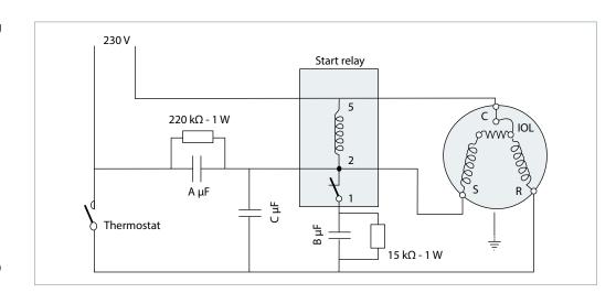
IOL Motor protector A & C Run capacitors B C Start capacitor
