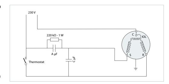
IOL Motor protector A & C C Run capacitors Common
