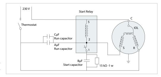
IOL Motor protector Run capacitors Start capacitor A+C В C Common
